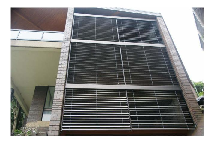
6/ The **SURE SHADE® Ultimate 120S** can be manufactured with wire guides if the wind loading is moderate and aesthetics of minimial visual obstruction is paramount. Since the 120S slat is inherently stable a higher wind loading can be accommodated when compared to the 100F or 80C constructed with wire guide.
